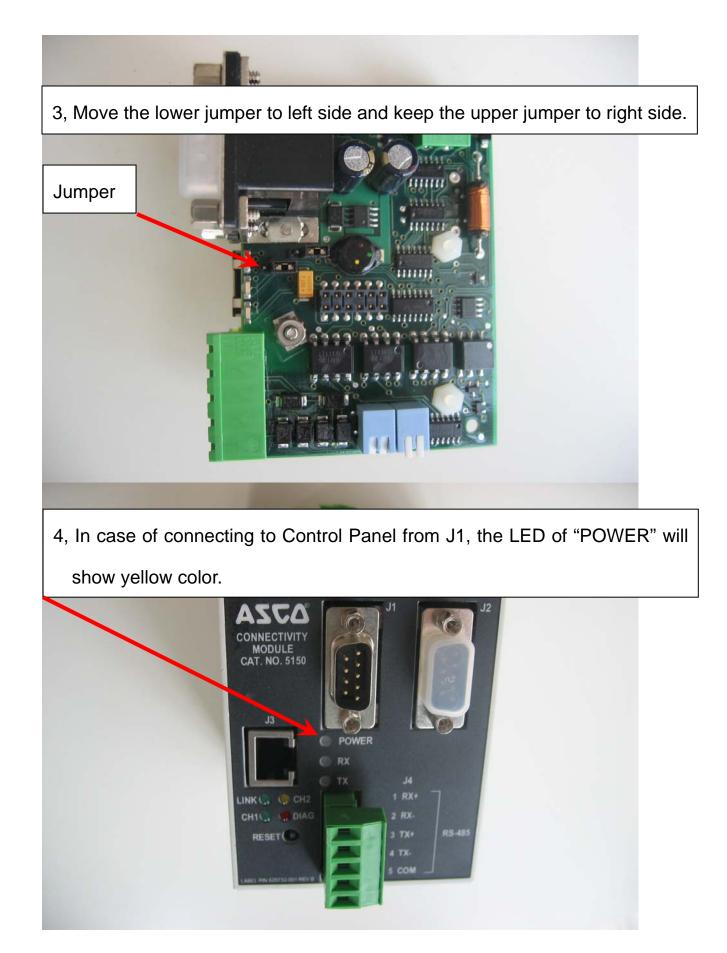
Tips: This module can work with either Ethernet function or Modbus function depending on the location of the lower jumper.
